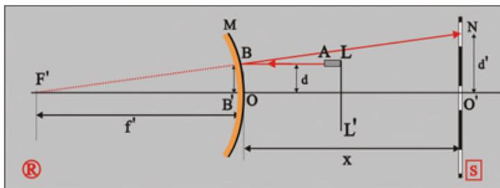
Figure 4: Schematic representation of the experimental setup.
