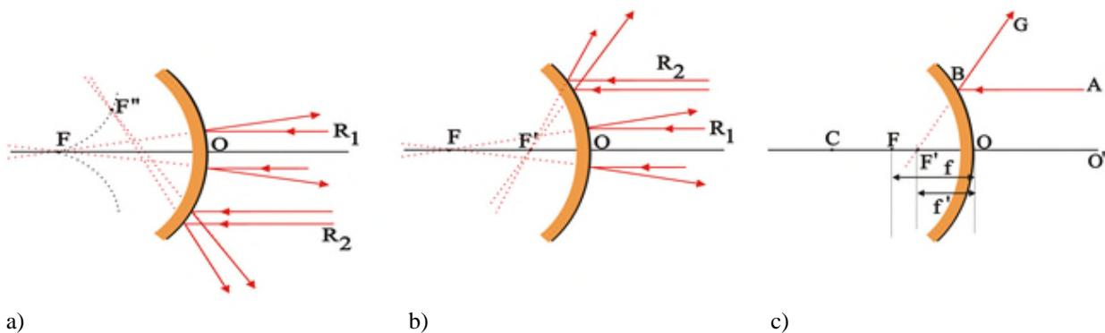
Figure 2: a) divergence of paraxial rays  $R_1$  and non-paraxial rays  $R_2$  incident on a convex mirror; b) the extension of the reflected ray AB (non-paraxial) intercepts the optical axis of the mirror at  $F'$  instead of the focus F; and c) foci of the paraxial (focal length  $f$ ) and non-paraxial rays  $R_1$  and  $R_2$  (focal length  $f'$ ).
