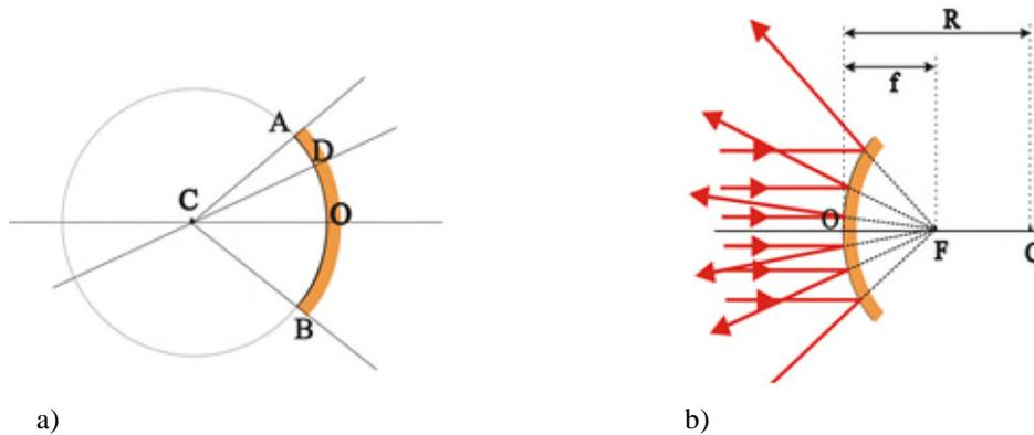
Figure 1: a) spherical mirror: CO is the optical axis, CD is a secondary axis; and b) the focal point F of an ideal convex mirror, which is defined by the reflection of parallel to the principal axis rays.
