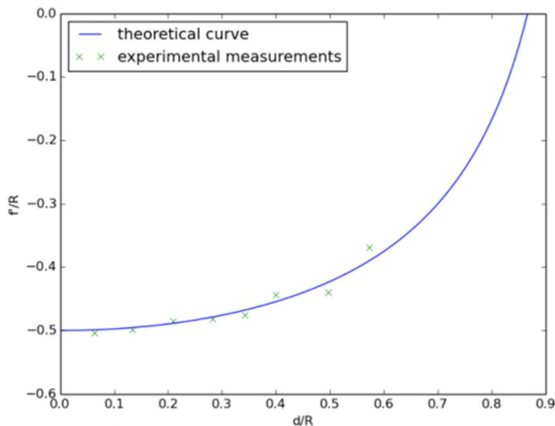
Figure 6: Plot of  $f'/R$  versus  $d/R$  for a convex mirror. The solid line is the theoretical curve and the discrete points are the experimental measurements.
